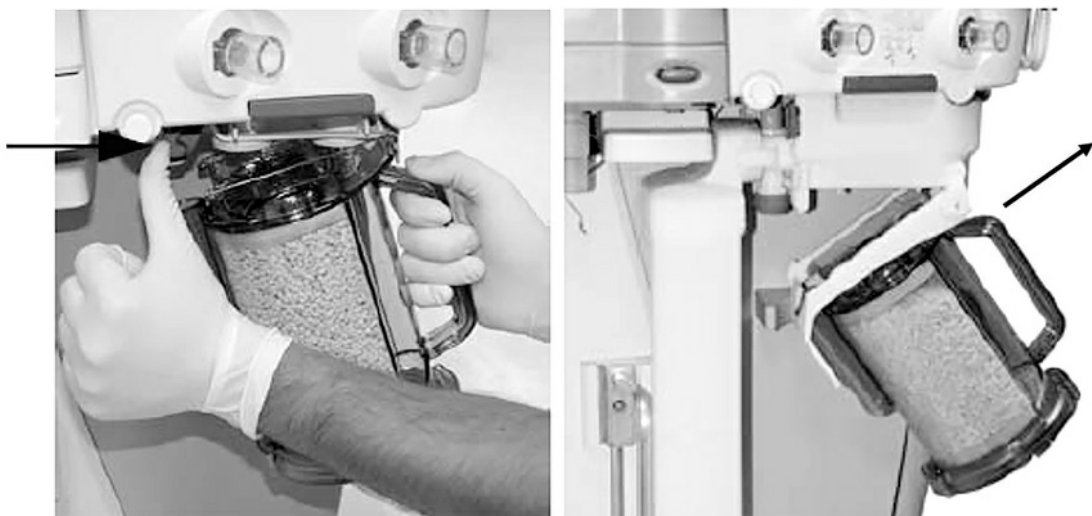
FIGURE 16.37 Changing carbon dioxide granules in the
