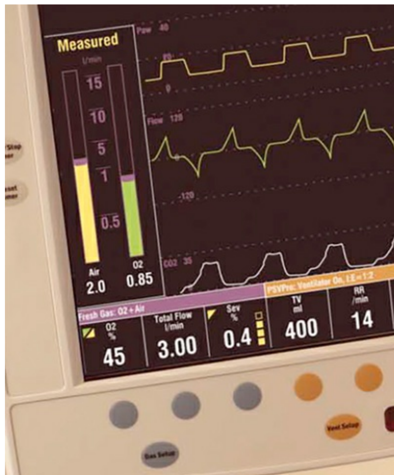
FIGURE 16.11 Electronic control of inspired oxygen, carrier gas, and total fresh gas flow, Aisys. (Courtesy GE Healthcare, Madison, WI.)
