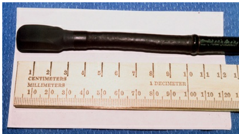
FIGURE 17.24 Transesophageal echocardiography probe. Distal tip contains thermistor and piezoelectric elements.
