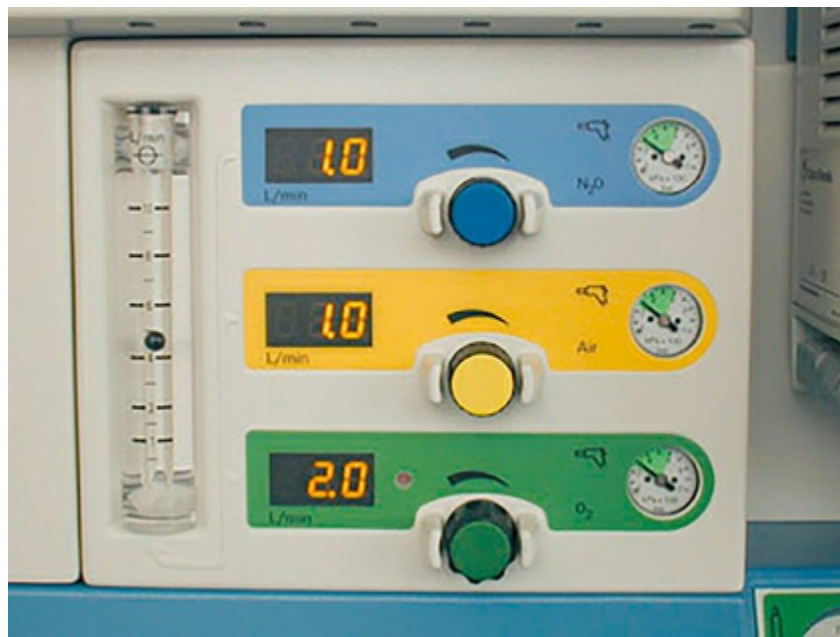
FIGURE 16.15 Flowmeters on the Fabius GS are arranged vertically. The oxygen knob ( at the bottom ) is different visually, and to touch, from control knobs for air and nitrous oxide. To the left of each flow-control knob is a digital display of flow and the common gas outlet flowmeter (glass tube); to the right is the pipeline pressure gauge for each gas. (Copyright Drägerwerk AG & Co. KGaA, Lubeck. All rights reserved.)
