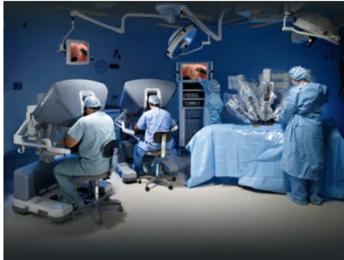
FIGURE 35.1 Surgeon operates while seated at the robotic console. (Courtesy of Intuitive Surgical Inc., Sunnyvale, CA.)
